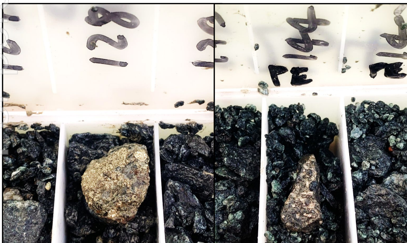
Figure 2 - Example of disseminated sulphides in RC chips from the Callisto discovery (patchy disseminated sulphide in NRC264, downhole depths as marked)
